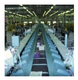
In most pick to conveyor systems cases must be sorted into outbound orders before they are palletized or loaded directly onto outbound trailer.
